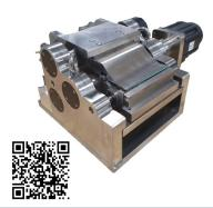
The Tridex PGS-100 Burr-Free Electrochemical Point Grinding System is a fully programmable pointing and material handling system that easily integrates with the Tridex SG-1645 or SG-2060 ECG Grinders. Using ECG, the PGS-100 manufactures a wide variety of medical device points on tubing or solid wire, such as medical needles or K-wires. The PGS-100 is capable of handling a wide amount of work pieces providing high throughput for specialty pointing applications.
