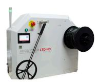
The Accu-Feed HPD High Performance Dereeler is designed for large spools and heavy gauge materials. Its large dancer arm, stronger drive transmission and revised part path eliminates reverse-bending during the feed process, which is ideal for olefin, Teflon®, and heavy gauge materials.
