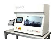
The SYNEO Accu-Lase V200 Automated UV Laser Processing System allows for greater process capability in precision tube cutting of polyimide tubing and complex hole making, as well as polymer marking. The V200 is a fully-automated laser micromachining system, allowing the operator to batch load parts, which are singularly picked up and fed by a vacuum pick head.
